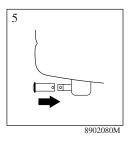
Refit the connector pin cover as in the illustration.
