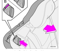
A - Catch in closed position B - Catch in open position
