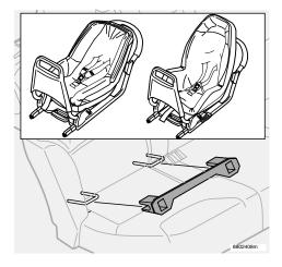
NOTE: Isofix attachment points are located on both outer rear seats. The rail can be moved from one side to the other as needed.
