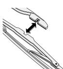
Press the entire wiper blade down so that the wiper arm eye passes through the hole in the wiper blade mounting.
