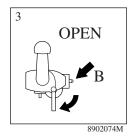
Remove the connector pin cover.
